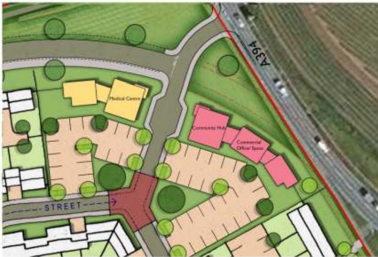
Sketch Layout of Surgery, community & commercial buildings with minimum 80 car parking spaces
